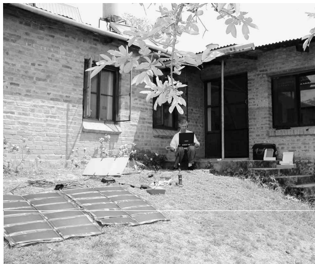
Fig 1 The SCT emergency pack in use at the Tansen Hospital in the western hills of Nepal. Solar panels provide the power for a digital camera, a laptop computer and a satellite telephone.
